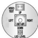
OSD CONTROL BOARD
