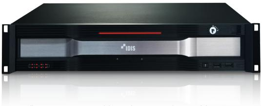
The IDIS Enterprise NVR, IR-300A, allows users to establish a reliable, high performance surveillance system in minutes while providing exceptional manageability. The IR-300A operating system (OS), powered by SSD and IDIS Solution Suite VMS, is perfect for large-scale systems and ensures important data retention through RAID and Redundant Power.
