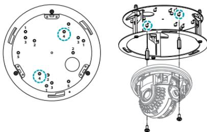
\*When using the screws of DC-D4233RX / DC-D4223RX models, combine the two as shown below.
