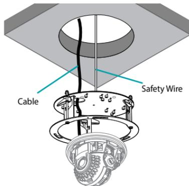
3 Mount the bracket to the ceiling, then fix it with the calmp (3-point) by turning the clamp screws clockwise.
