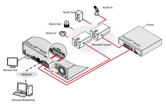
DirectlP $^{\text{TM}}$  NVR makes it easy to use cameras without extra network configurations. Each camera can be controlled via the DirectlP $^{\text{TM}}$  NVR setup menu, without any PC. For detailed camera settings, please see the camera setting pages of DirectlP $^{\text{TM}}$  NVR manual.
