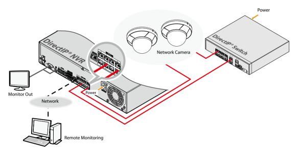
DirectIP<sup>®</sup> NVR makes it easy to use cameras without extra network configurations. Each camera can be controlled via the DirectIP<sup>®</sup> NVR setup menu, without any PC. For detailed camera settings, please see the camera setting pages of DirectIP<sup>®</sup> NVR manual.
