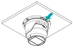
5 The top cover rotates on the bottom cover and is tightened. As shown in the picture, align the markings on the bottom cover and the top cover of the main body and join them.
