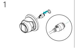
Insert a round rubber ring (silicone rubber) into the RJ45 jack.
