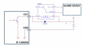
I (In): Connect an alarm-in device to this port. (Mechanism: Choose between an NC (Normally Closed) type or an NO (Normally Open) type) → Connect a mechanical or electrical switch to the alarm in port and the GND (ground) connector. Alarm in range is 0V to 5V. In order to detect alarm input from an electrical switch, the signal must be higher than 4.3V from an NC switch or less than 0.3V from an NO switch and must last for longer than 0.5 seconds.
