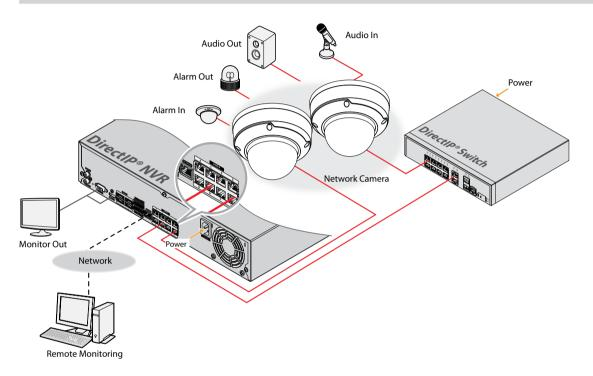
DirectIP® NVR makes it easy to use cameras without extra network configurations. Each camera can be controlled via the DirectIP® NVR setup menu, without any PC. For detailed camera settings, please see the camera setting pages of DirectIP® NVR manual.
