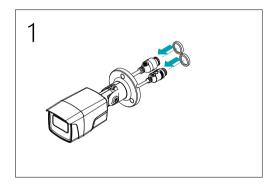
Insert a round rubber ring (silicone rubber) into the PoE IN jack and PoE OUT jack each.
