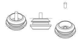
2 Insert the LAN cable through the cable rubber using the protect connector.
