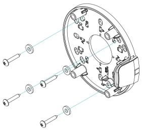
**7** Screw the junction box to installation plate by using screws provided with the camera.
