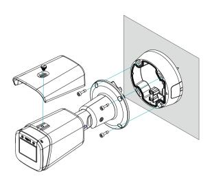
12 Band the stand to adjust the camera angle accordingly. For details, refer to the <u>Angle</u> <u>Adjustment</u>.
