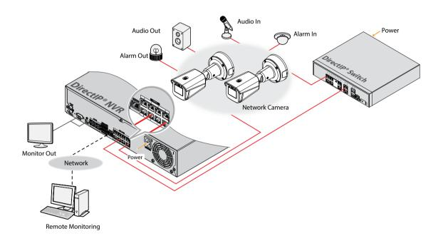
DirectIP® NVR makes it easy to use cameras without extra network configurations. Each camera can be controlled via the DirectIP® NVR setup menu, without any PC. For detailed camera settings, please see the camera setting pages of DirectIP® NVR manual.
