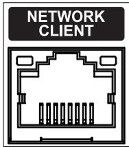
This NVR is capable of connecting to networks via an ethernet connector. Connect an RJ-45 cable (Cat5, Cat5e, or Cat6) to the NVR's network port. It's possible to operate and upgrade the NVR remotely over a network. For more information on ethernet connection setup, refer to **Network Setup in the operation manual**.
