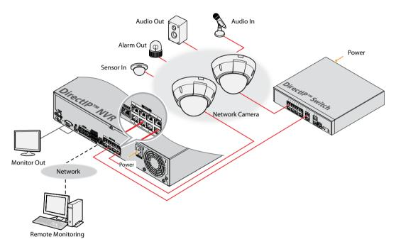
DirectIP<sup>TM</sup> NVR makes it easy to use cameras without extra network configurations. Each camera can be controlled via the DirectIP<sup>TM</sup> NVR setup menu, without any PC. For detailed camera settings, please see the camera setting pages of DirectIP<sup>TM</sup> NVR manual.
