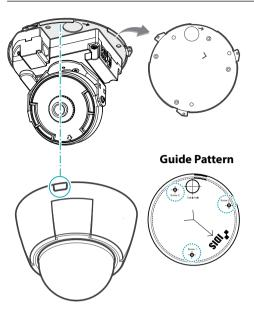
1 Use the screws provided with the camera to secure the bottom cover on a wall or a ceiling.
