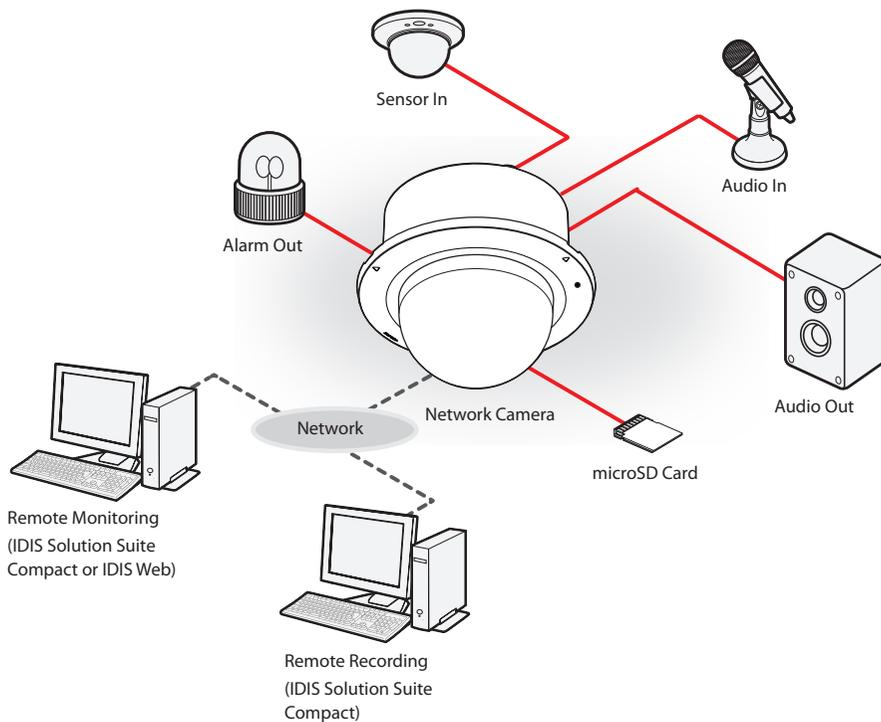
Control the camera over the network from software installed on a computer.
