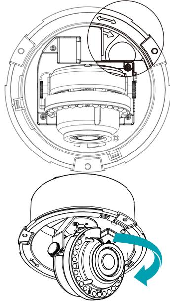
8 Adjust the angle of the lens. For more information, refer to the **Angle Adjustment**.
