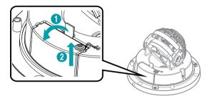
Insert a SD memory card into the SD memory card slot with the 'micro SD' print facing upward.
