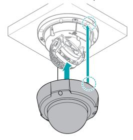
2 Fasten the screws for the dome cover clockwise using the allen wrench provided with the camera.
