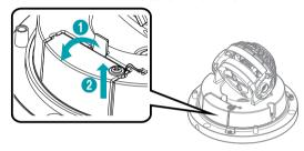
2 Attach the enclosed desiccant in the SD memory card slot cover to prevent moisture.
