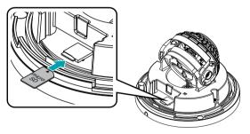
Push the SD memory card until it disengages from the slot, and then pull it out.
