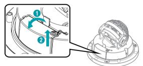
2 Insert a SD memory card into the SD memory card slot with the 'micro SD' print facing upward.
