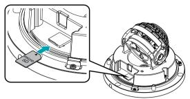
Push the SD memory card until it disengages from the slot, and then pull it out.
