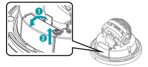
2 Insert a SD memory card into the SD memory card slot with the 'micro SD' print facing upward.
