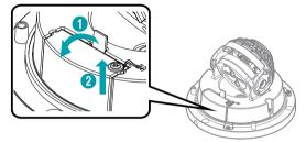
2 Attach the enclosed desiccant in the SD memory card slot cover to prevent moisture.
