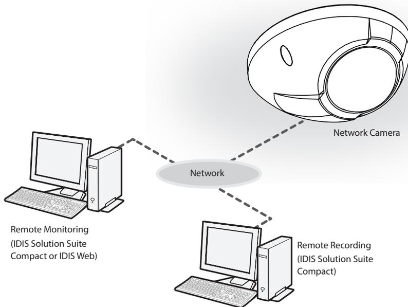
Control the camera over the network from software installed on a computer.
