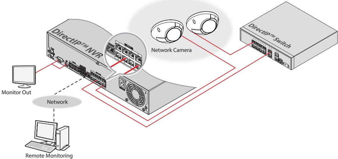
DirectIP™ NVR makes it easy to use cameras without extra network configurations. Each camera can be controlled via the DirectIP™ NVR setup menu, without any PC. For detailed camera settings, please see the camera setting pages of DirectIP™ NVR manual.
