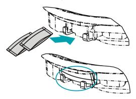
After you insert the SD memory card in the camera, secure the body on a wall or ceiling using the screws and anchors that came with the camera.
