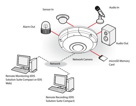
Control the camera over the network from software installed on a computer. Ideal for using the camera over the network from a remote location.
