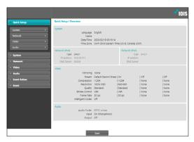
From the Remote Setup screen, select the menu on the left to display the current settings. Select an option under the menu to change the corresponding settings. Once you have changed the settings, click **Save** to apply the settings.
