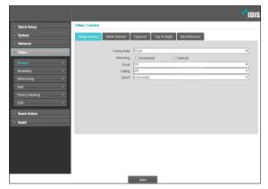
• Frame Rate: Set the frame rate of image sesor. Streaming settings are reset when changing the frame rate.
