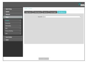
• Smart IR: Prevent the object from being saturated by IR light. Select **Auto** to control saturation only when the zone is over-saturated.
