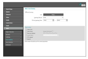
Line: Click Setup and define the line and the conditions for which each line crossing event will occur up to 8 conditions.
