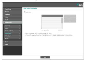
List: Displays a list of audio files to playback. Click Add or Remove to add/remove audio files. Select an audio file from the list and then click Play to listen to the file. The total audio file upload capacity is 8MB.
