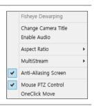
• Enable Audio: Enables audio transmission with remote locales. Select to display Select buttons.
