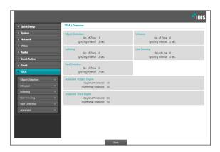
Configure IDLA (IDIS Deep Learning Analytics) settings. It quickly detects objects (human, cars, and bikes) and faces, and based on them, object detection, intrusion, loitering, line crossing, and face detection are performed.
