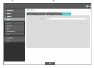
Smart IR: Prevent the object from being saturated by IR light. Select Auto to control saturation only when the zone is over-saturated.
