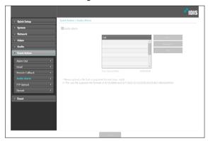
List: Displays a list of audio files to playback. Click Add or Remove to add/remove audio files. Select an audio file from the list and then click Play to listen to the file. The total audio file upload capacity is 8MB.
