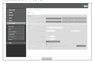
• FTP Server: Click Add to register a new FTP server. Click Remove to remove a registered FTP server. When an event is detected, a .jpg image of the event detected image is uploaded to the Primary Server. If the upload to the Primary Server fails, the file will be uploaded to the Secondary Server. Upload to the Secondary Server will continue to be attempted until successful. Fill out the fields below and click Test to test the FTP server connection settings. Once the test is complete, click OK.
