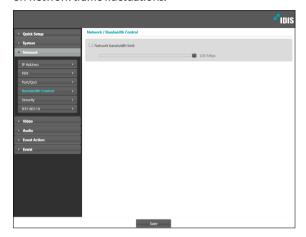
Select **Network Bandwidth limit** and then specify the maximum bandwidth. The camera will not be able to use more than the specified limit in the event of network traffic.
