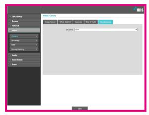
• Smart IR: Set the brightness of the IR LED.
