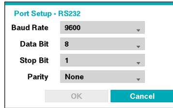
Configure the port's setting based on the PTZ camera manufacturer's instructions.
