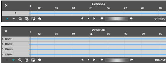
Recording date and time are shown on the top of the search window. The indicator line on Record Table indicates the current playback position. Use the arrow buttons on the remote control to move the current playback position in units of individual sectors. Alternatively, use the mouse to jump to the desired playback position.
