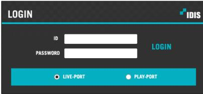
If connecting by entering <http://web.idisglobal.com>, enter the DVR's IP address in the Device Address field. Selecting the Use FEN Service option on the login window allows you to enter the DVR name registered to the FEN server instead of its IP address. You will be prompted to enter the FEN server's address and port number under Setup.
