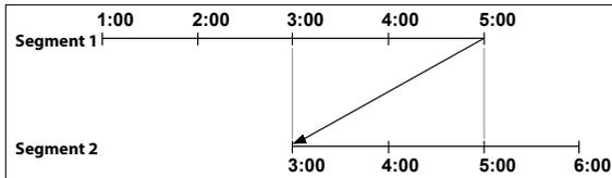
When searching overlapped video recordings, you can choose a specific point in time or a time frame. If you use the **Go to the Date/Time** option and select a point within the overlapped time period (**4 o'clock**, for example), you must specify **4 o'clock** in which of the two existing segments.
