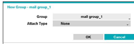
A virtual keyboard appears allowing you to enter the Group name. You can select among CBF, JPG, and MP4. When selecting CBF, the DVR will attach an event detected video clip to an email. When selecting JPG, the DVR will attach the event detected image file (JPEG format) to an email. When selecting MP4, the DVR will attach the event detected video clip (MP4 format) to an email.
