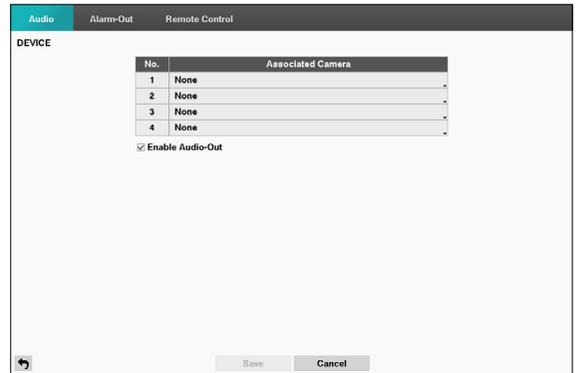
The DVR can record up to four audio inputs. A list of cameras appears, and you can select which camera you want associated with that audio input.
