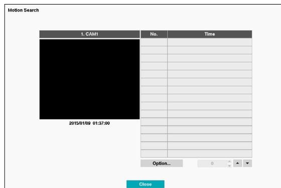
Motion Search cannot be performed while using a split screen layout. Select Single Screen mode.
