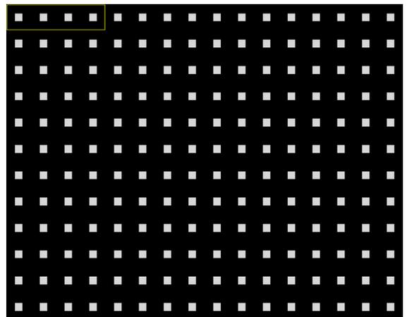
Use the remote control's arrow buttons to move the block selection window up, down, left, and right. The selection window consists of 4 blocks per row. Select/deselect individual blocks using the **Camera** buttons. You can use the mouse to drag the zone and then select, clear, or reverse the selection.
