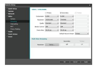
Primary, Secondary, Tertiary: Multistreaming is supported. (priority: Primary > Secondary > Tertiary).
