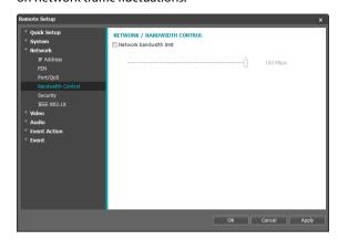
Select **Network Bandwidth limit** and then specify the maximum bandwidth. The camera will not be able to use more than the specified limit in the event of network traffic.
