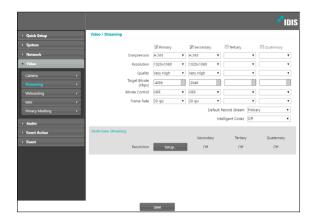
Primary/Secondary/Tertiary/Quaternary: Multistreaming is supported (priority: Primary > Secondary > Tertiary > Quaternary). Enable/disable streaming use. The lower stream settings may change depending on higher stream settings. The tertiary and quaternary streams may not be available depending on higher stream settings. (refer to the table below).
