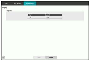
Connect the spot monitor using the BNC cable. Select the box in the **Channels** column.
