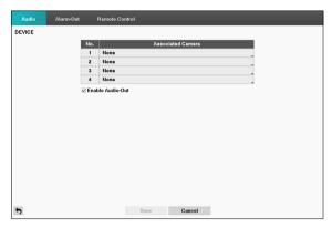
The DVR can record up to four audio inputs. A list of cameras appears, and you can select which camera you want associated with that audio input.
