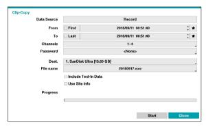
Channels: Specify which channel to save the recording to.
