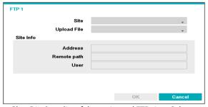
Site: Display a list of the registered FTP sites. Select an FTP site from the list. If the Use setting of the NetFS site is set to other than ALL or Clip-Copy, you cannot select the FTP site. You can change the Use setting or register other FTP sites in the NetFS setup screen on the Network menu.
