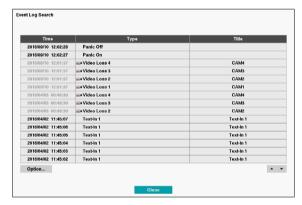
Select an event to display the recording made on the selected time and date (paused state). Select the Play button in the middle of the screen to start playing back the recording. Use the screen form to load recordings from other cameras.
