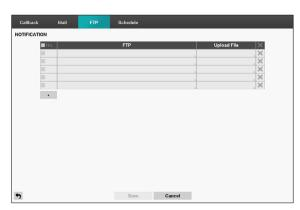
The FTP feature uploads event detected image or video clip on the FTP site when an event occurs. Select the + icon at the bottom of the list to add a FTP site.
