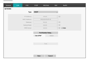
Select **DHCP** and then **Save** to retrieve IP address and other network settings automatically from the DHCP server. Once the network settings have been retrieved, the DVR's current IP address is displayed in the IP Address field.
