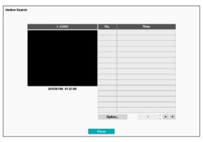
Motion Search cannot be performed while using a split screen layout. Select Single Screen mode.
