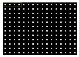
Use the remote control's arrow buttons to move the block selection window up, down, left, and right. The selection window consists of 4 blocks per row. Select/ deselect individual blocks using the **Camera** buttons. You can use the mouse to drag the zone and then select, clear, or reverse the selection.
