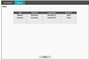
Configure Disk Bad and Disk Temperature settings under **Setup > System > System Event**.
