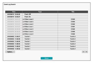
Select an event to display the recording made on the selected time and date (paused state). Select the Play button in the middle of the screen to start playing back the recording. Use the screen form to load recordings from other cameras.
