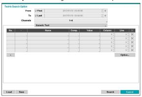
Select First under From and Last under To to search the recording from start to finish. Alternatively, you can uncheck the First and Last options and specify the search time frame manually.
