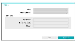
Site: Display a list of the registered FTP sites. Select an FTP site from the list. If the Use setting of the NetFS site is set to other than ALL or Clip-Copy, you cannot select the FTP site. You can change the Use setting or register other FTP sites in the NetFS setup screen on the Network menu.
