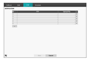
The FTP feature uploads event detected image or video clip on the FTP site when an event occurs. Select the + icon at the bottom of the list to add a FTP site.
