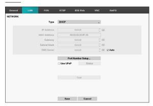
Select **DHCP** and then **Save** to retrieve IP address and other network settings automatically from the DHCP server. Once the network settings have been retrieved, the DVR's current IP address is displayed in the IP Address field.
