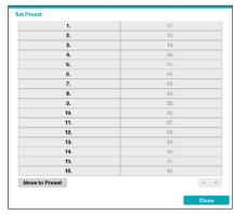
While in PTZ mode, select the **PRESET SELECT** button on the remote control to display the **Move to Preset** window. Select a preset to move the current PTZ camera to the selected preset's position.
