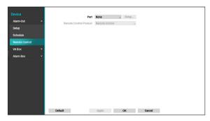
Port: Select None, RS232 or RS485. Click the Setup button and then select the correct Baud Rate,
