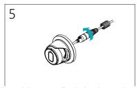
Push the waterproof cap body and cap into the RJ45 jack and rotate it.
