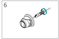
Lock the waterproof cap into the waterproof cap 6 body.
