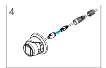
Δ Connect the plug terminal to the RJ45 jack.
