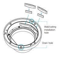
Before closing the dome cover, make sure that the gasket ring is securely fixed.
