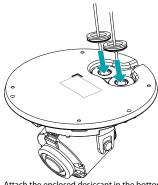
Attach the enclosed desiccant in the bottom to prevent moisture.
