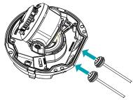
6 Attach the enclosed desiccant folding in half in the bottom to prevent moisture.
