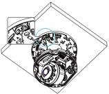
8 Attach the camera body to the installation bracket by rotating it clockwise as shown below. You will hear a click when it is properly mounted.
