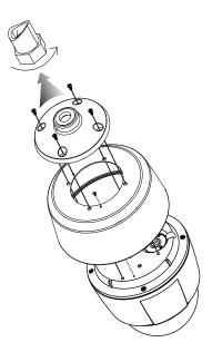
Remove the install screw from the camera body.
