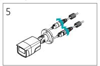
5 Push the waterproof cap body and cap into the PoE IN jack and PoE OUT jack each and rotate them.
