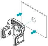
3 Remove the guide shape from the bracket using a nipper or other tools.
