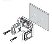
3 Assemble the camera to the bracket by turing it to the desired direction. Fix the camera using left and right screws and connect cable.
