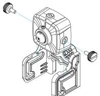
2 Remove a sheet on the double-sided tape on the bracket, and attach the bracket to a wall by matching the hole.
