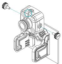
4 Fix the main unit to a wall or ceiling using screws.
