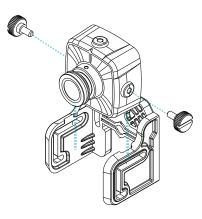
2 Fix the bracket to a wall or ceiling using double-sided tape or screws.
