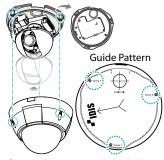
1 Use the screws provided with the camera to secure the bottom cover on a wall or a ceiling.
