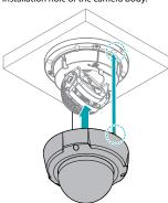
2 Fasten the screws for the dome cover clockwise using the allen wrench.
