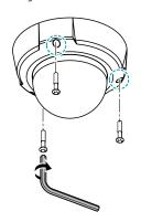
Attach the dome cover to the bottom cover. Press the area where the triangular mark meets the dome cover assembly hook to assemble the dome cover.
