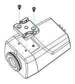
Install the bracket on the top or the bottom of the camera to secure it. For bracket installation, use 1/4-20 UNC (20 Thread), 2.5mm +/- 0.2mm (ISO standard), or 0.197 (ASA Standard) standard screws.
