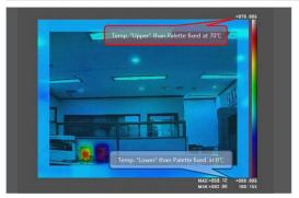
The maximum temperature of the palette, 70°C, is displayed in white, the top color of the palette, and the minimum temperature of 0°C, the palette, is displayed in purple, the lowest color of the palette. Colors between 70°C and 0°C are represented by colors between white and purple to match the ratio of 70°C difference.
