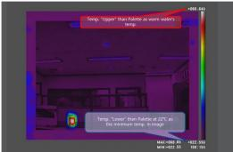
The maximum temperature of the pallet, 62°C, is displayed in white, the top color of the palette, and the minimum temperature of 22°C, the palette, is displayed in purple, the lowest color of the palette. Colors between 62°C and 22°C are represented by colors between white and purple to match the ratio of 40°C difference.
