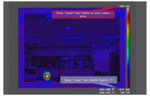
White color is displayed on the cup with 62°C temperature - the highest one in the pallet. The minimum temperature of the pallet, 17°C, is displayed in purple at the bottom of the pallet. Colors between 62°C and 17°Care represented by colors between white and purple to match the ratio of 45°C difference.
