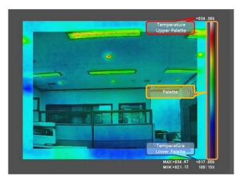
Screen with 'WhiteRainbow' pallet. Color of thermal image is displayed from range of the pallet -from the color on the top is the highest temperature to the lowest temperature's color at the pallet's bottom. The highest temperature of the pallet whith color which is 34°C. The lowest one of the pallet is violet, 17°C. Color between 17°C and 34°C are displayed by colors between white and violet.
